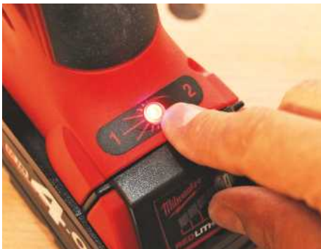
▲ This button alters the jigsaw's speed; two speeds are available
